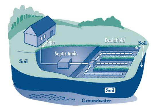
Septic tanks must be designed to accommodate the wastewater flow generated in the building(s) they serve. If not, the wastewater will not remain in the tank long enough to allow the removal of settleable solids. Without sufficient time for settlement, or if the tank is not regularly pumped out, solids may be flushed into the soil absorption system, where they may cause clogging and, ultimately, failure of the system.
